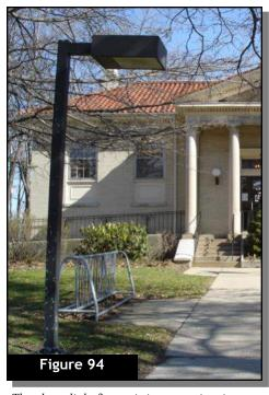
The above light fixture is inappropriate in scale and height for this pedestrian application.
